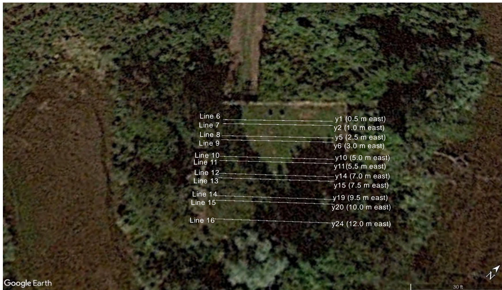
Figure 4. Location of GPR transect lines using 500 MHz antenna, and where they overlay the 12 x 12 m grid.
